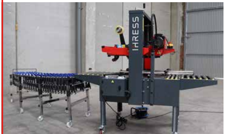
Extensible free wheels outfeed conveyor from 1,2 m to 4,8 m
